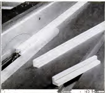
bottom edge of the miter cut. Remove waste stock between the kerfs with additional passes of the saw. Make the splines from \frac{1}{2} "-square hardwood strips. Adjust the table and rip fence for undercuts that will form an L-shaped cross-section by clearing out a \frac{1}{4} "-square rabbet. After applying glue, align the mitered edges and drive the splines into place. END
